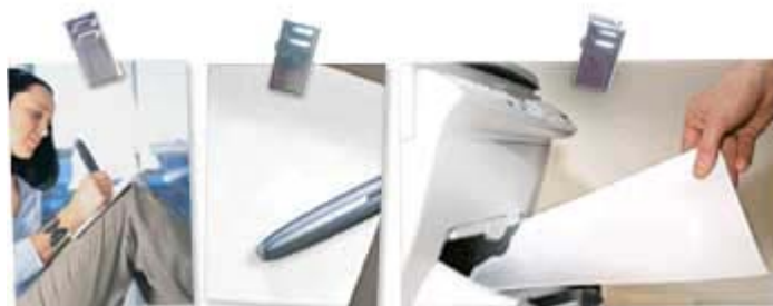
Fig.5: The Anoto pen-paper system to support annotation
