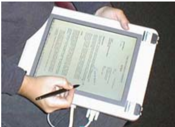
Fig.2: XLibris pen-tablet display system
